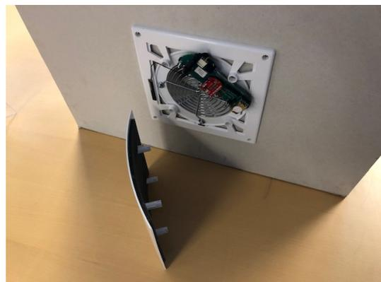
*Fig 4 - Fan cartridge (from stale air side)*
